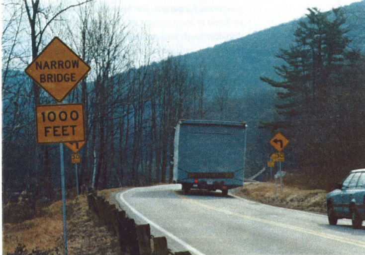
Figure 2: Oversize Load Encroaching into Opposing Lane and Shoulder 1
